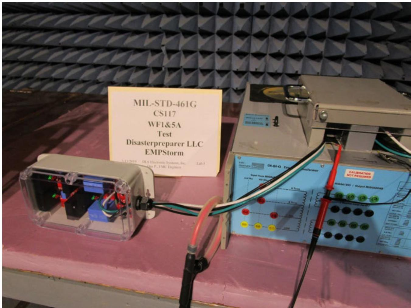
CS117 WF1 and WF5A Test
