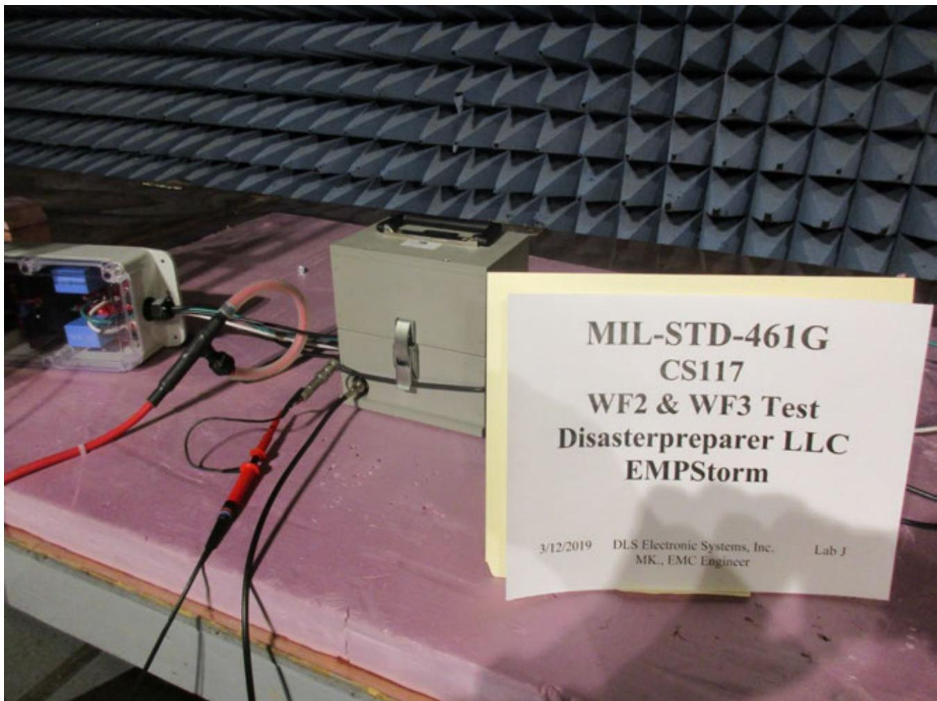
**CS117 WF2 and WF3 Test**
